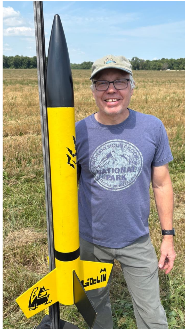
Randy Jenkins puts his 3X scratch-built "Goblin" on the launch pad. He flew it with a Research I245 motor and it took it to an altitude of 2400 feet.
