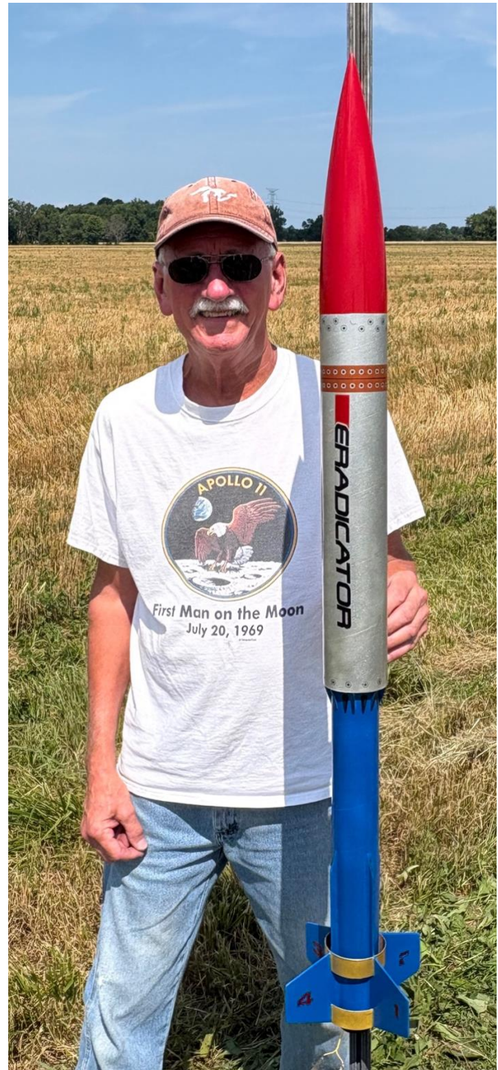
Mark Fickenscher takes his Sirius rocketry "Eradicator" rocket out to the launch line. He flew it with an AT G64 motor to an altitude of 2200 feet
