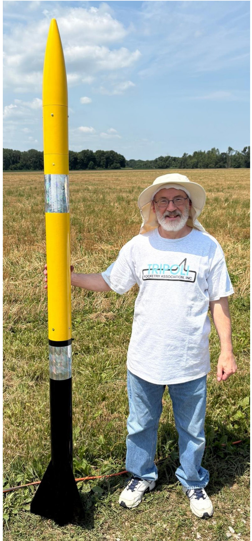
Neal Bade does his first flight of the day with a LOC/Precision "HyperLOC 835" that flew to 1400 feet with an AT I161 motor.
