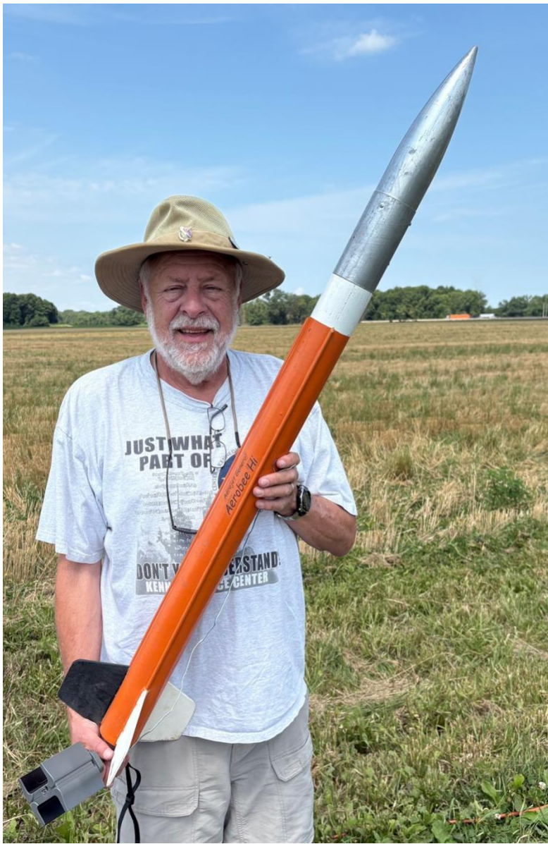
Mark Hanna with his scratch-built "Aerobee Hi" rocket. He flew it with a CTI G84 motor to an altitude of 1500 feet.
