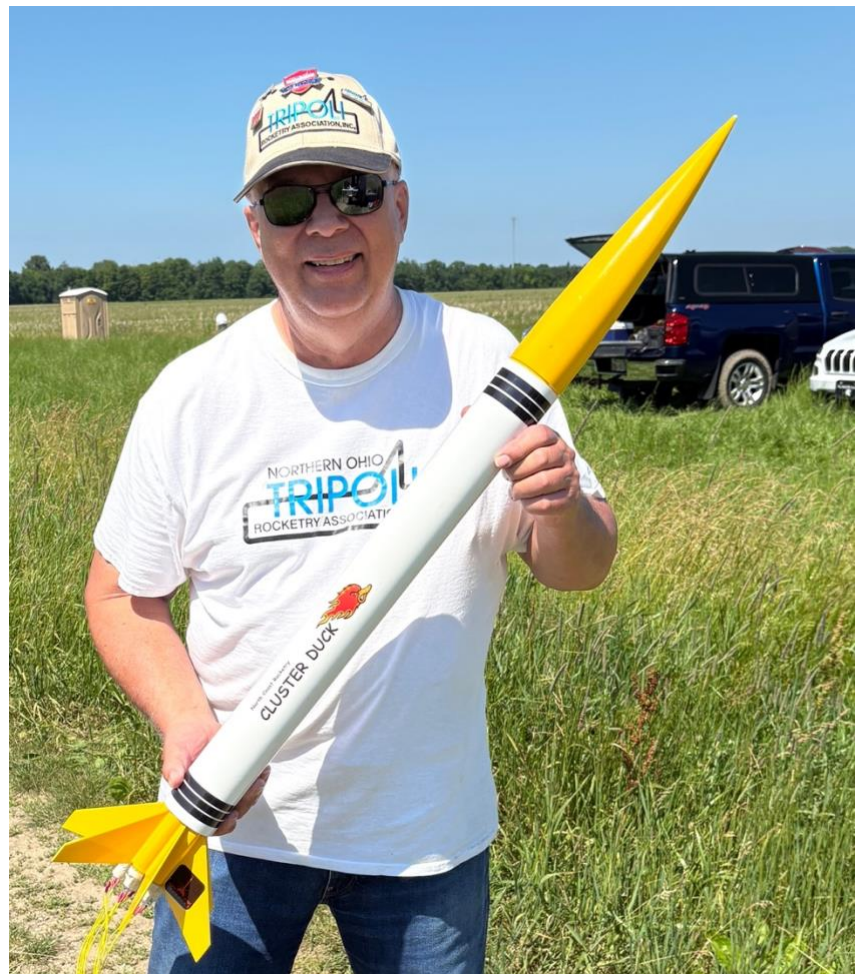
Chris Pearson flew his North Coast Rocketry "Cluster Duck" (again!) with a cluster of six Estes C6 motors and an E12 (which didn't cat to this time!) to an altitude of 1000 feet. Old-school flashbulb/thermalite ignition got all the motors ignited.
