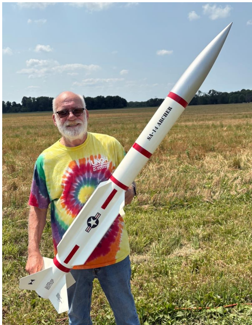
Frank McGroarty shows his original 4" North Coast Rocketry "Archer SA-14" that he flew with an AT G74 motor. It was underpowered and would have flown better with a high-thrust H motor.
