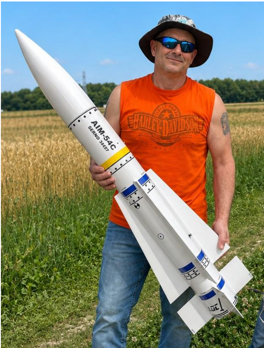
Dennis Calo heads out to the launch pads with his LOC/Precision 4" "Phoenix". He flew it with an AT I180W to an altitude of 2200 feet.
