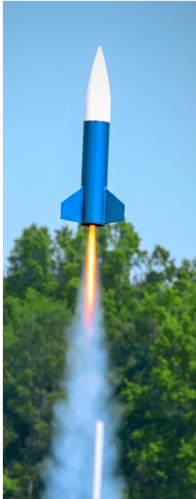
Frank McGroarty takes his LOC/Precision "Warlock" to the pad for his TRA Level 2 certification flight. He flew it with a 38mm CTI J290 motor, which unfortunately cato'ed about 500 feet off the ground.
