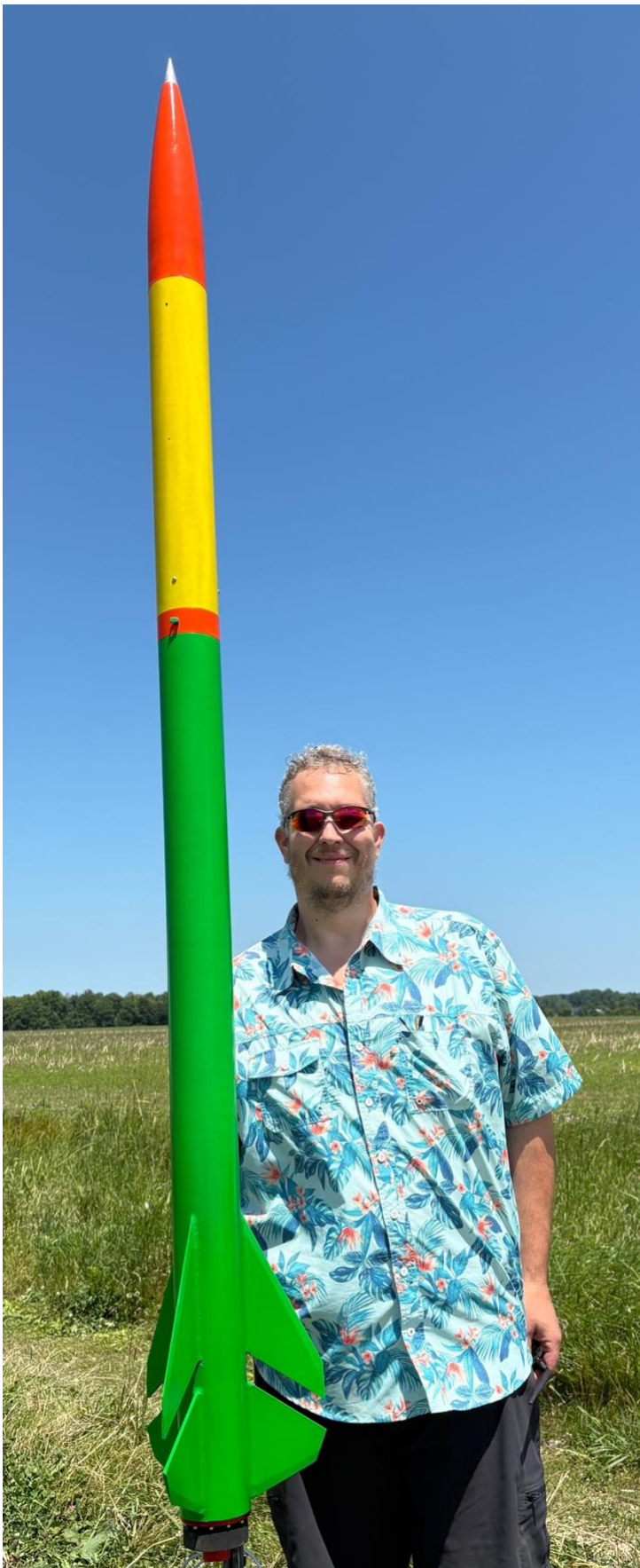
Mike was expecting an altitude of 4000 feet but the rocket had a lot of tip-off and only got to about 2000 feet.
