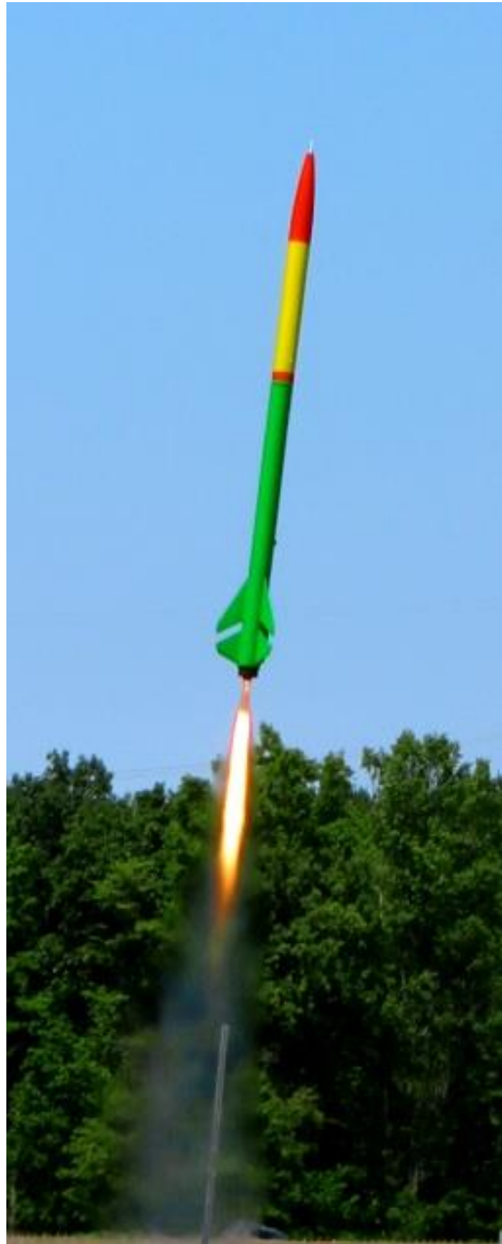
Mike was expecting an altitude of 4000 feet but the rocket had a lot of tip-off and only got to about 2000 feet.
