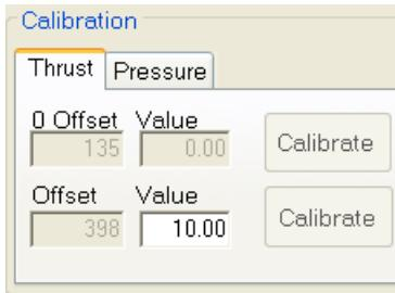
With no weight on the load cell in appropriate orientation (horizontal or vertical) click the top Calibrate button, next to *Value*=0.00. This will set *0 Offset* to whatever value the load cell produces without weight. It will show a number and that is what the computer will reference as *Value*=0.00.
