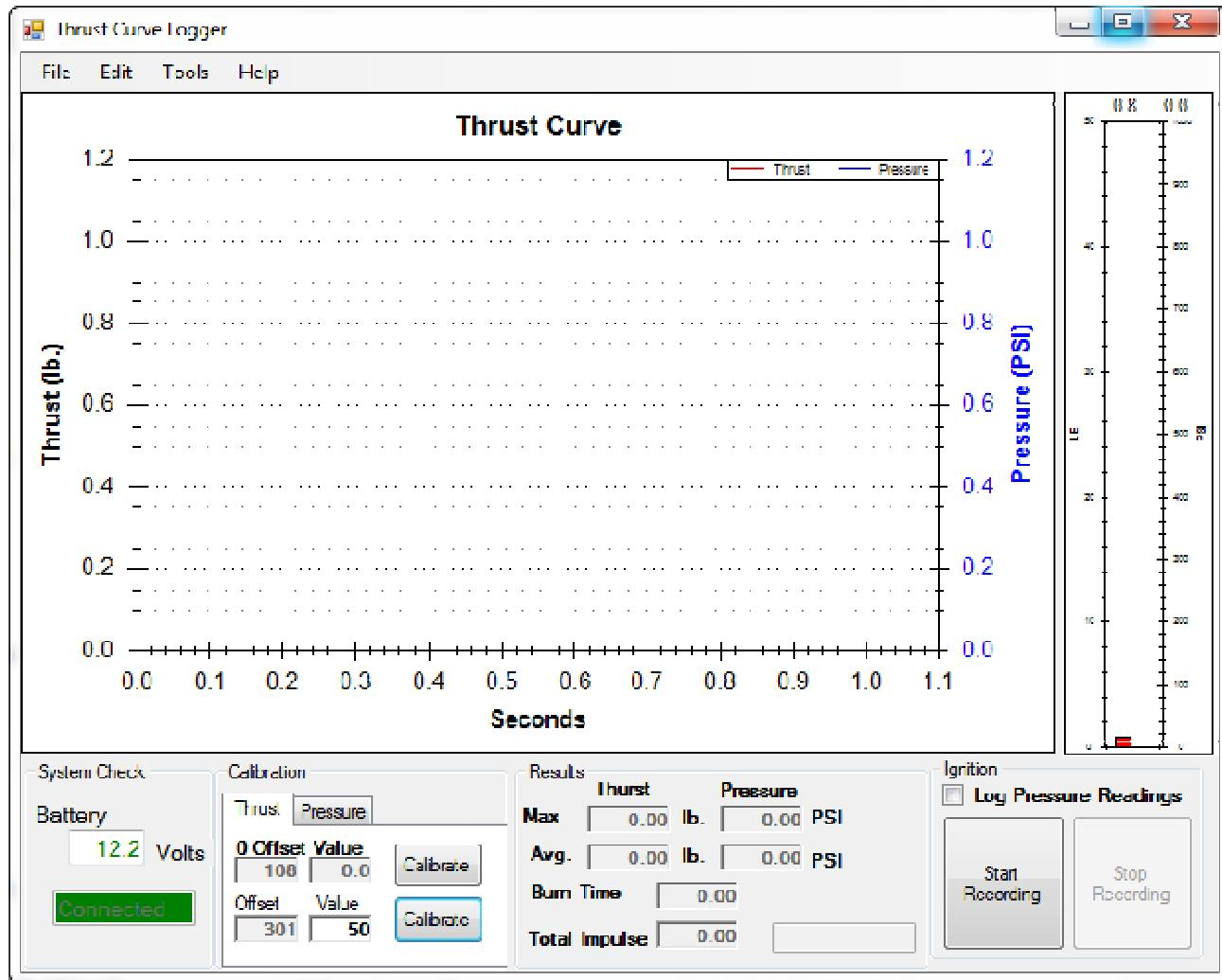
When the screen opens you should see, in the System Check box (lower left corner) these values showing the battery voltage and if you are connected to the Interface Box (green), if you're not (Red).
