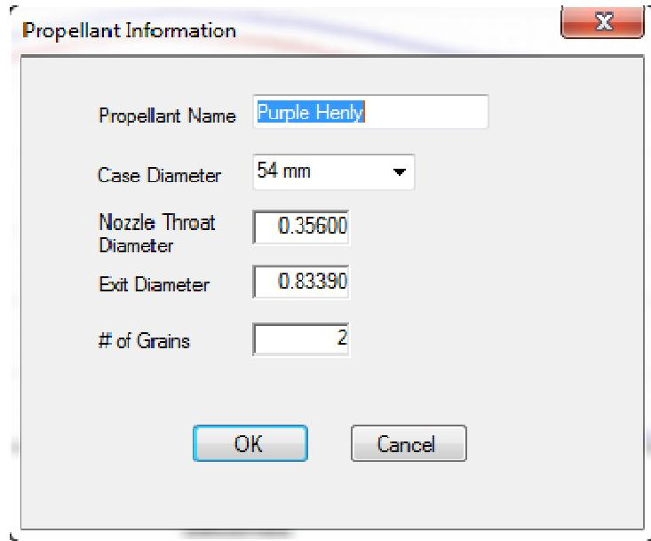
Whether firing a Test Motor or a Flight Motor you should fill out the requested data fields. This data is optional but will be very useful later when characterizing the propellant. Once you click OK this window will close and the logger will start collecting data. You will see the Red and Blue chart lines searching along the Time Line looking for data. In the case of Flight Motors only the Red line will be seen.
