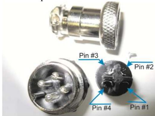
The Pressure Transducer has three(3) Pins as shown in the photo.
