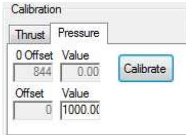
Enter the maximum value for the pressure sensor that you are using into the lower *Value* field. Then press the Calibrate button. Each day you use the system the Pressure Calibrate button should be clicked to adjust for the current atmospheric pressure.
