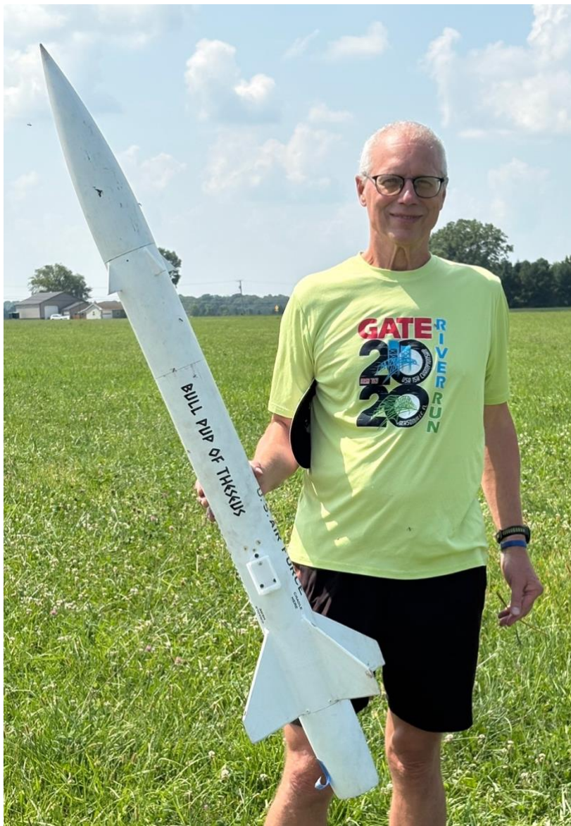
Chip Jenkins flew his scratch-built "Bull Pup" with a Research H220 motor using NASSA K2 Fast propellant to an altitude of 1900 feet.
