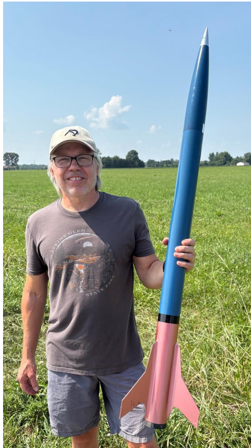
Randy Jenkins poses with his OBH "Steampunk" that he flew with a Research H220 motor using NASSA K2 Fast propellant which took it up to an altitude of 2400 feet.
