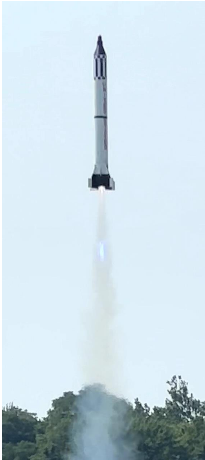
Mark Hanna's scratch-built 6" diameter Mercury Redstone lifts-off on the power of an AT J460 motor. The rocket achieved an altitude of 1350 feet.
