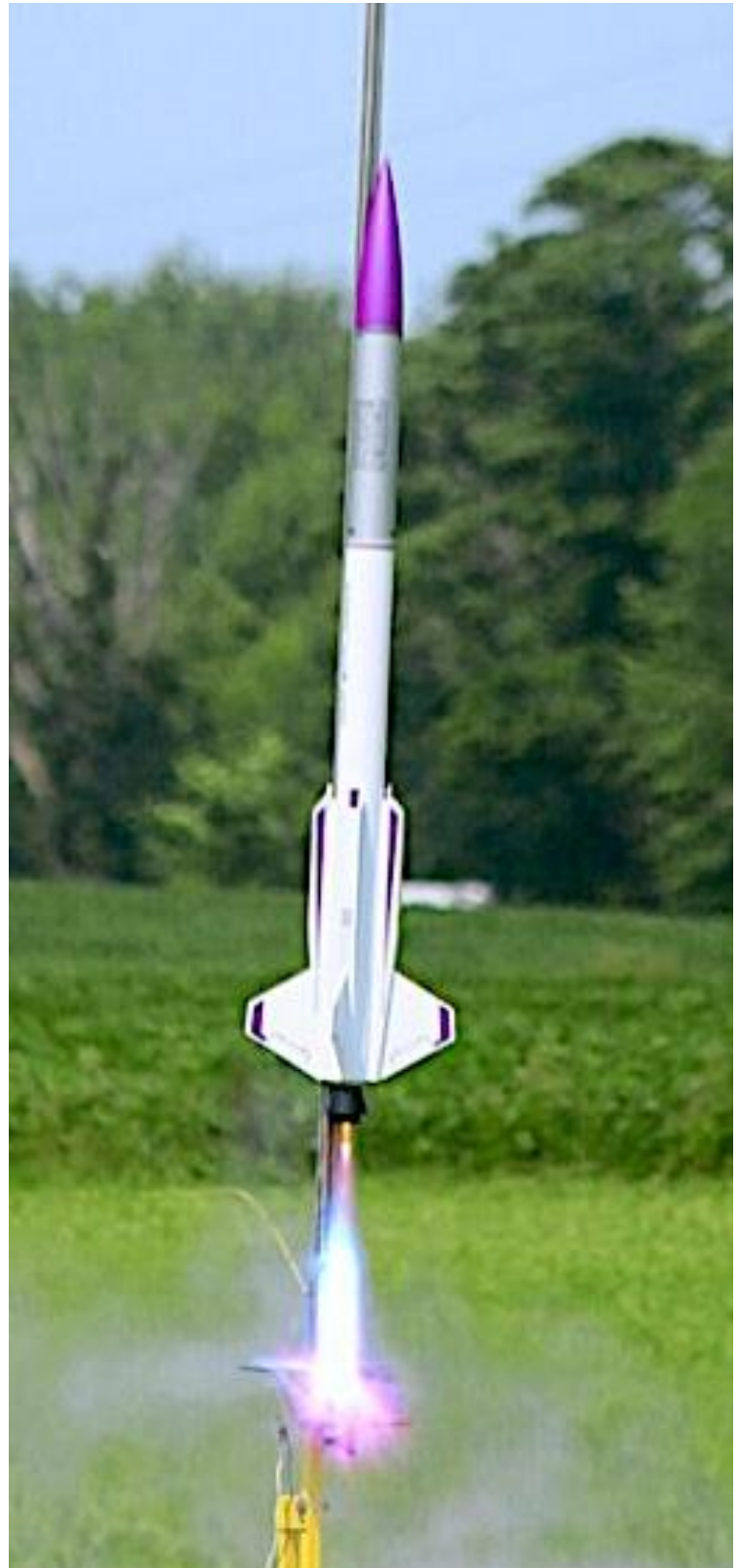
Catherine Calo with her Bad Boy Rocketry "QCC Explorer" that she certified L1 with at last month's launch. This time she flew it with an AT H220T motor. A Chute Release brought it back close to the pads.
