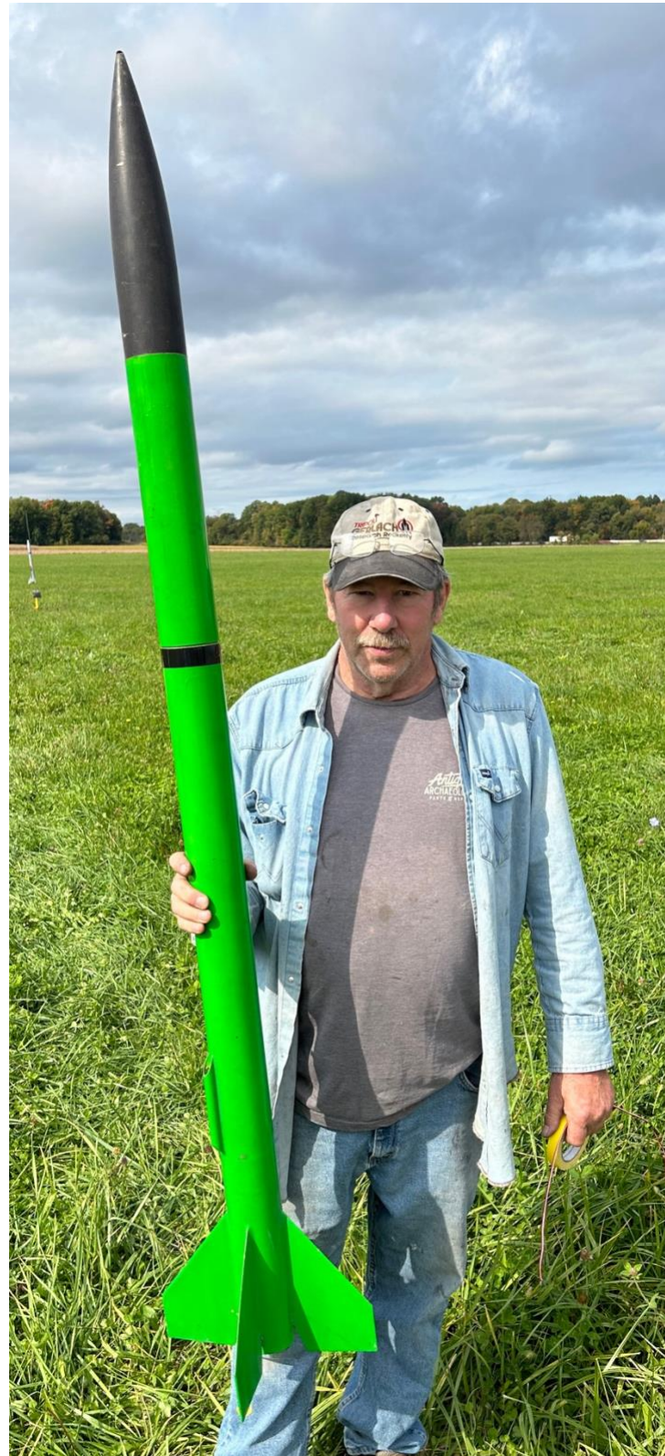
Steve Eves with his scratch-built "Green Machine" which he flew with a Research I141 motor to an altitude of 1800 feet.
