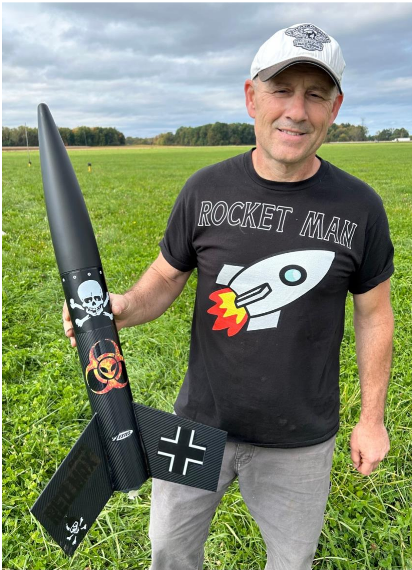
Dennis Calo heading out to the launch pad with his Estes "Big Der Red Max", done up in a carbon fiber wrap. He flew it with an AT F26FJ motor.
